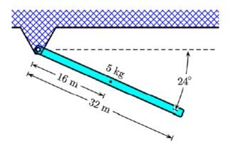
What is the angular acceleration of the rod immediately after it is released? The moment of inertia of a rod about the center of mass is  $\frac{1}{12} m L^2$ , where *m* is the mass of the rod and *L* is the length of the rod. The moment of inertia of a rod about either end is  $\frac{1}{3} m L^2$ , and the acceleration of gravity is  $9.8 \text{ m/s}^2$ .
